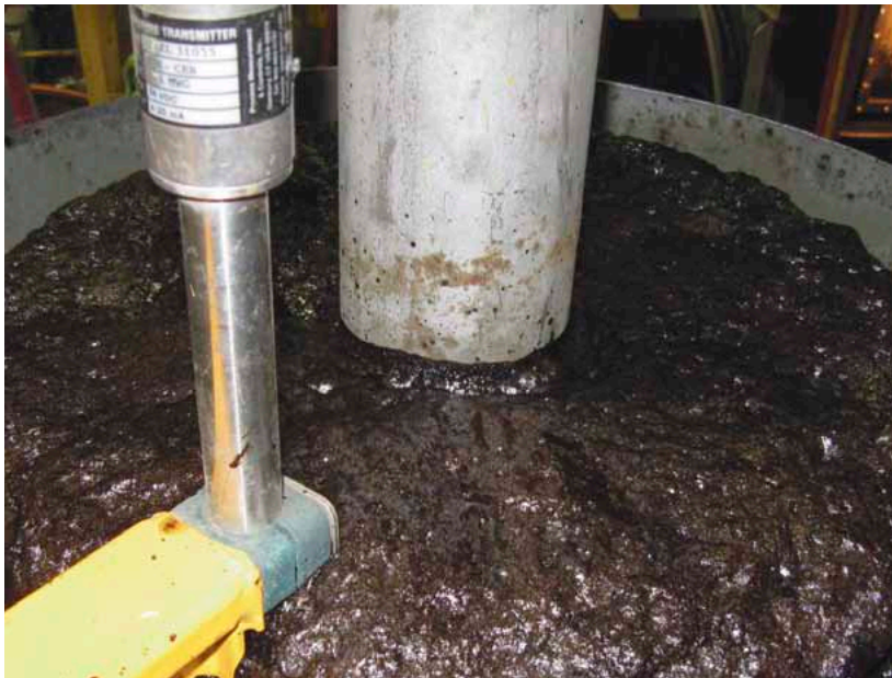
Jameson Cell lab scale flotation test of oil sands (top), and phosphate (below)
