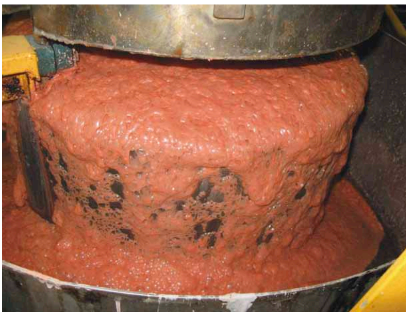
Jameson Cell lab scale flotation test of oil sands (top), and phosphate (below)
